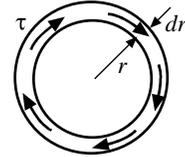
$$T = \int_0^R \frac{\mu\omega 2\pi}{h} r^3 dr = \frac{2\pi\mu\omega}{h} \frac{R^4}{4} = \frac{\pi \times 2.36 \times 10^{-5} \times \frac{400 \times 2\pi}{60} \times (3/12)^4}{2 \times 0.08/12} = \underline{91 \times 10^{-5} \text{ ft}\cdot\text{lb.}}$$
