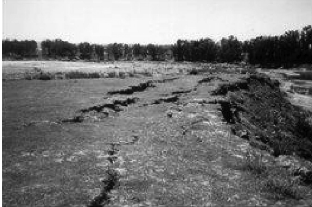
Figure 2.26 Lateral spreading (El Asnam, 1980).
