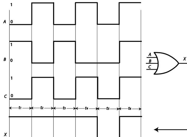
Solution 2.16: With the C input is 1, the OR gate output will remain 1 regardless of what is occurring at the other inputs. Because any HIGH input will keep an OR gate output high. Therefore, the glitch will not appear in the output.
