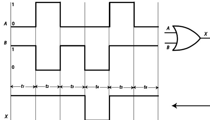
Solution 2.15: The OR gate output is determined by realizing that it will be HIGH whenever any of the three inputs is at a HIGH level. Thus, in the timing diagram, the fifth time interval is low, rest are high.
