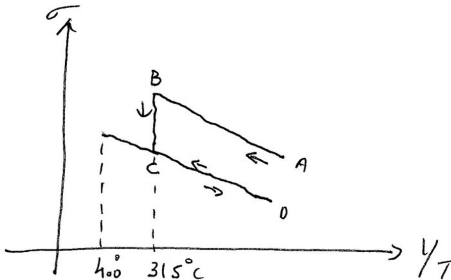
From  $A \rightarrow B$ ,  $WO_3$  film is in amorphous state. From  $B \rightarrow C$ ,  $WO_3$  film is transitioning to polycrystalline. From  $C \rightarrow D$ ,  $WO_3$  film is in polycrystalline state. It is irreversible. Once the film is polycrystalline, it cannot go back to being amorphous.  $WO_3$  becomes polycrystalline at  $315^\circ C$ .
