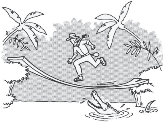
FIGURE 2.4 Structural requisites: structure with adequate strength but excessive flexibility. (From A.J. McDonald, Structure and Architecture , Architectural Press, London, p. 20, 2001. With permission.)
