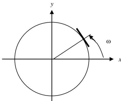
Hour angle  $\omega$  is the angle the Earth has rotated since solar noon. For simplicity, we show the case  $\omega > 0$  (i.e. in the afternoon).
