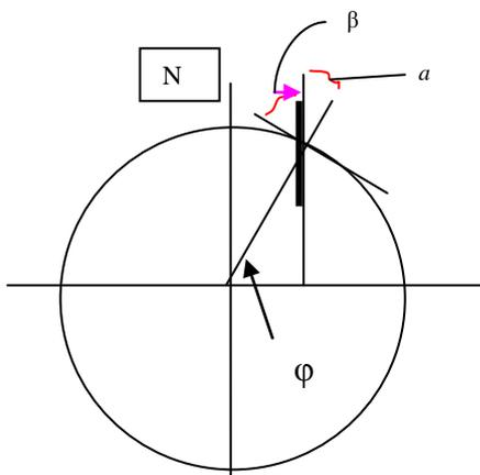
We work through this diagram to establish that the plane of the collector (thick line) is normal to that of the equator. Angles  $\beta$  and  $\phi$  are given as indicated.
